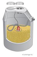
Pneumatic pickup Filler neck Access and maintenance hatch
