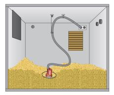
Safety valve Impact protection mat Ladder & hatches Filler neck Pneumatic pickup
