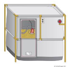
Integrated impact protection mat / Access and maintenance hatch / Sun Pellet Mole extraction system / Pellet dispensing line / Filler neck / Air feedback system / Dust-tight fabric / Watertight base tub
