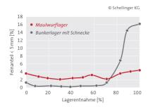
Low pellet segregation and amount of fine material. This avoids disruptions to the supply system and in combustion.
